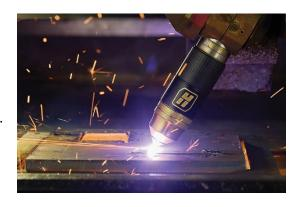
name a few. With the addition of 80A and 130A bevel cutting capabilities, cartridge now covers six mild steel cutting processes: 80A, 130A, 260A standard and bevel cutting.
