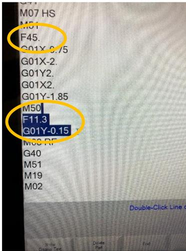
F45 = 45ipm speed through the cut for 0.75in (~19mm) material
