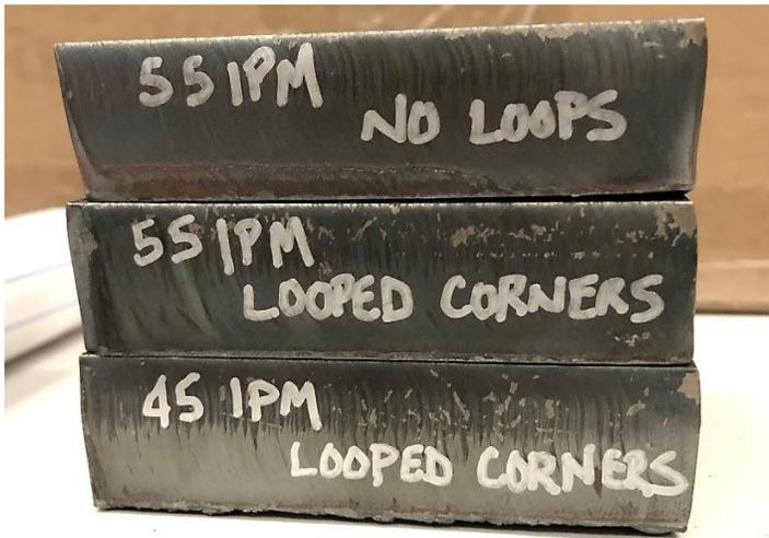
For 0.75in (~19mm) mild steel, the aluminum cut chart in the XPR manual (809830) calls for a speed of 45ipm. Increasing the speed to 55ipm yielded less dross and equivalent cut straightness.
