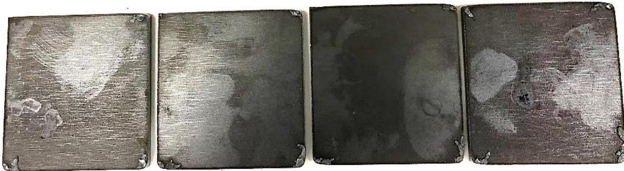
The above image shows the back of the cut parts. As you can see, there is very little dross. Any dross that does accumulate is easily removed.
