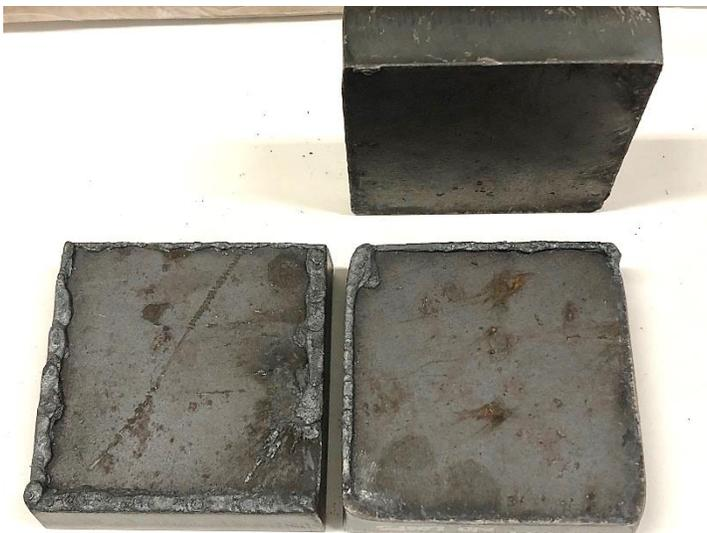
Bottom side view of dross on 0.75in (~19mm) cuts.
