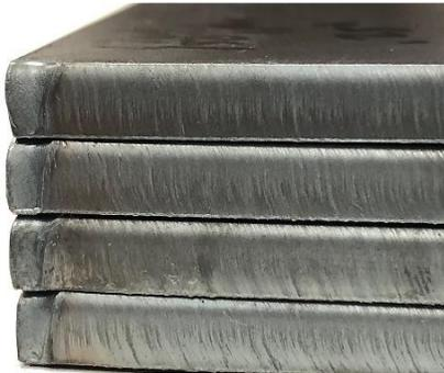
0.25in (~6mm) speeds top to bottom: 150ipm, 175ipm, 190ipm, 210ipm
