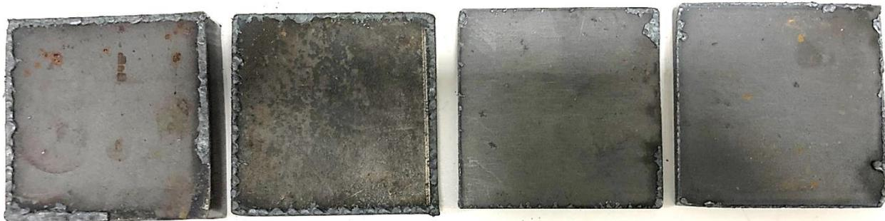
From left to right: The back of the cut parts, 0.75in (~19mm), 0.5in (~12mm), 0.25in (~6mm) 130A, and 0.25 (~6mm) 45A. You can see the presence of dross, however, it is not heavy and easily removed by hand.
